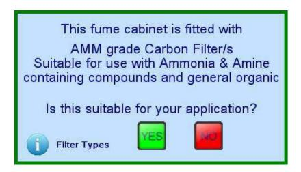
If the procedures carried out inside the cabinet are always the same this screen can be bypassed in the Supervisor Settings (see page11) When the filter type has been accepted the normal running screen below is displayed.
