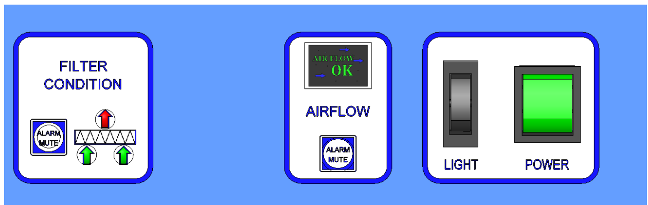
CONTROL PANEL With Airflow Monitoring and Filter Condition Monitoring
